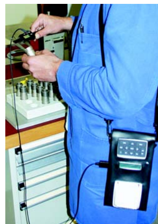
The above illustration shows the use of the Statistics Printer in the Transport Bag MSP 2t
